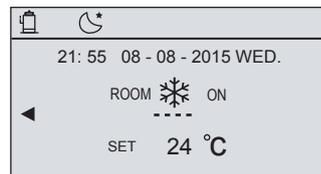
If application 4 (refer to 8.4 Application 4) is applied, please set WATER FLOW TEMP. to NON, and set ROOM TEMP. to YES, then the room temperature will be displayed on the home page, and the room temperature will work as the target temperature. The target outlet water temperature can be calculated from the climate related curves.
