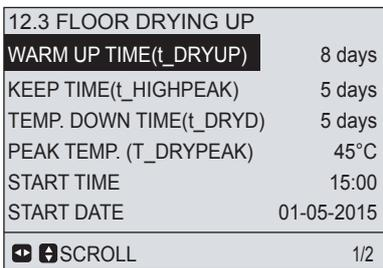
When the cursor is on **WARM UP TIME (t\_DRYUP)**, **KEEP TIME (t\_HIGHPEAK)**, **TEMP. DOWN TIME (t\_DRYD)**, **PEAK TEMP. (T\_DRYPEAK)**, **START TIME** or **START DATA**, Use ◀ ▶ and ▼ ▲ to scroll and adjust the parameter.
