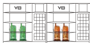
Continue operating in case of failure of one unit
