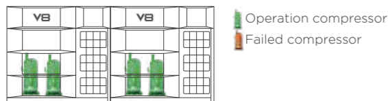
Intelligent load-bearing between units during normal operation
